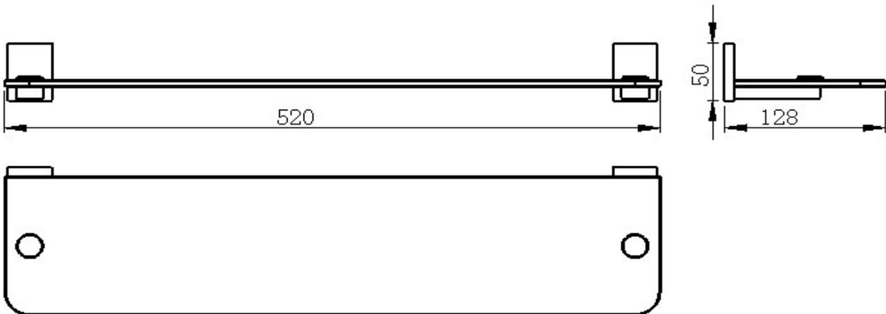
Dimensions: All measurements are in millimeters and are subject to normal manufacturing variations.
